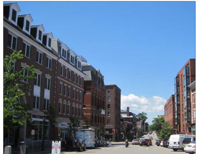
Roofs and roof lines shall avoid long unbroken expanses through the use of dormers, chimneys and changes in ridge line.
